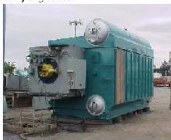
Gambar 28. Packaged Tube Boiler (Sumber: Perry Vldex)
